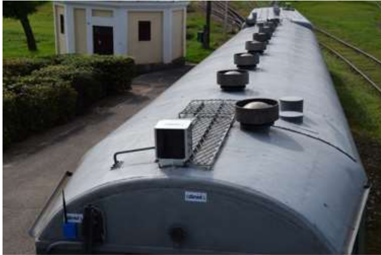
Figure 9-15: DEWI Project energy harvesting system
