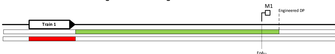
Figure 59: EoA with engineered D_DP, Full Moving Block
