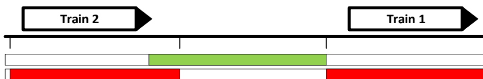
Figure 13: One Train Following Another – Fixed Virtual Blocks
