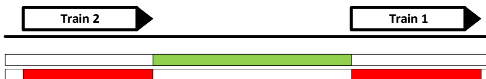
Figure 12: One Train Following Another – Full Moving Block
